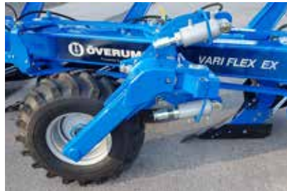
Side Mounted Combi wheel - 320/65x16 VFCXP, DX, EX & Vario Flex EX mid mounted
