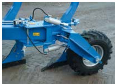
Hydraulic depth control for combi-wheel above
