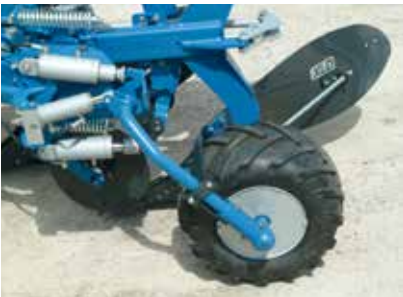
Hydraulic depth control and rim sides for tractor treaded support wheel.
