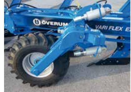
New side mounted combi wheel - 11.5-80 15.3 EX, VFEX, VFEX On-land. Choice of mechanical or hydraulic depth adjustment, hydraulic brake.
